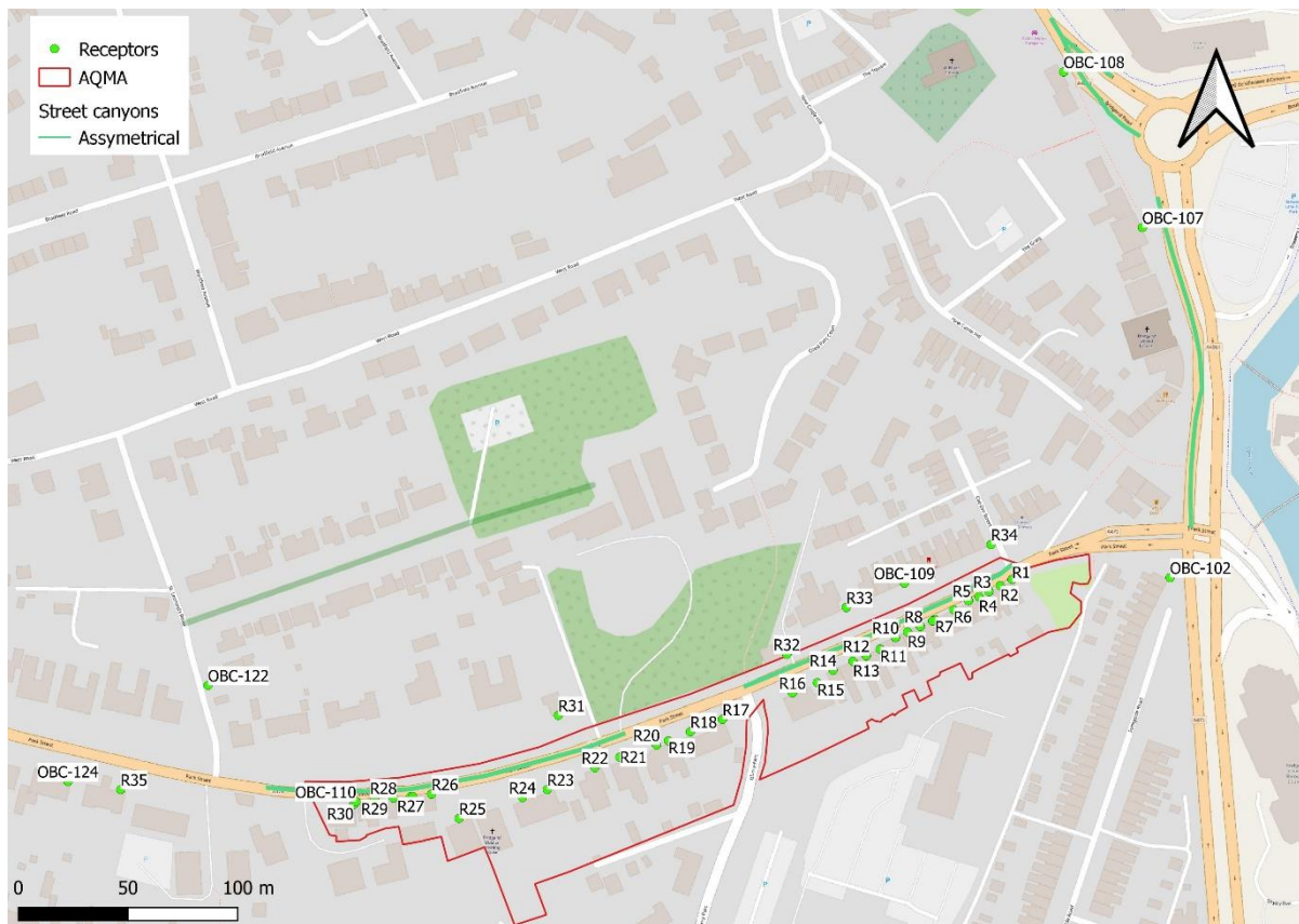
Figure 15 Street canyons in Bridgend
